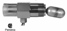
**LS200** Liquid Level Switches with 2" NPT mounting are float activated to operate an electrical SPDT snap switch (optional DPDT on some models) for alarm or shutdown of an engine or electric motor. The LS200 connects directly into the vessel wall and can be used with a weld collar (P/N 15050375) or Murphy external float chamber. L1100 models (1-1/2" NPT) are also available.
